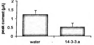
Fig. 1: CaCl activity in Xenopus oocytes. Currents were recorded using two-electrode voltage clamp. Oocytes were clamped at -90 mV and stepped in +10 mV increments starting at -50 mV. Bath solution was ND-96 + 1.8 mM Ca2+. Ten mM Ni blocked the Cl- current, which is calcium-dependent. Data on the left are means ± S.E.M.
