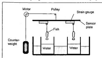
Figure 1. Simplified pictorial drawing of weighing apparatus. Fish (2 of 4 shown) are suspended by threads, and raised from the water by the stepping motor lifting the sensor plate under computer control. The external bath is temperature-controlled. Not shown is the pantograph which constrains the sensor plate to remain level, and the computer and its connections.
