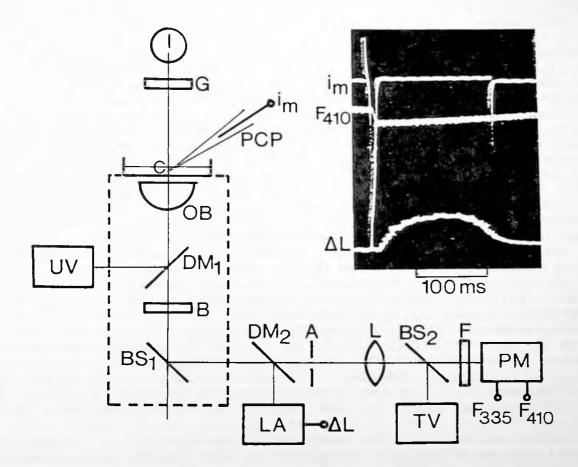
Figure 1. Simultaneous measurements of fluorescence signals (F335 and F410) and cell shortening (L). The diagrammatic representation shows the optical axis in a thin line. For details, refer to text. The inset panel shows sample traces of the membrane current  $(i_m)$ , the fura-2 fluorescence measured with excitation at 410 nm (F410) and the cell shortening (L). A decrease in F410) corresponds to an increase in the intracellular Ca<sup>2+</sup> activity.
